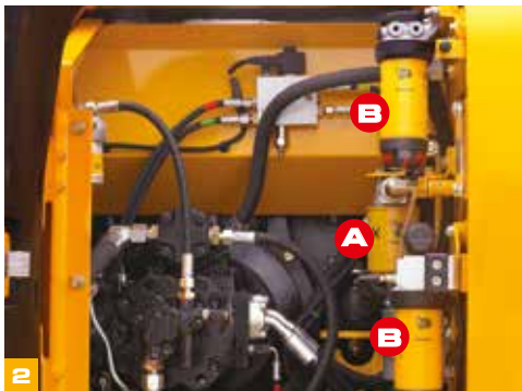
(A) Hydraulics oil filters (B) Fuel filters
